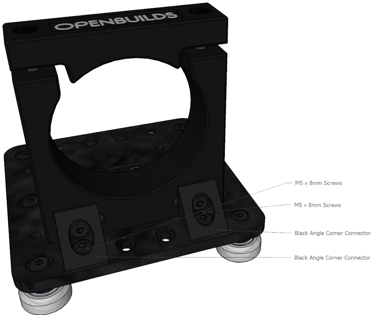
Figure 11: Assemble Z Axis Gantry Plate: Install Corner Connectors
