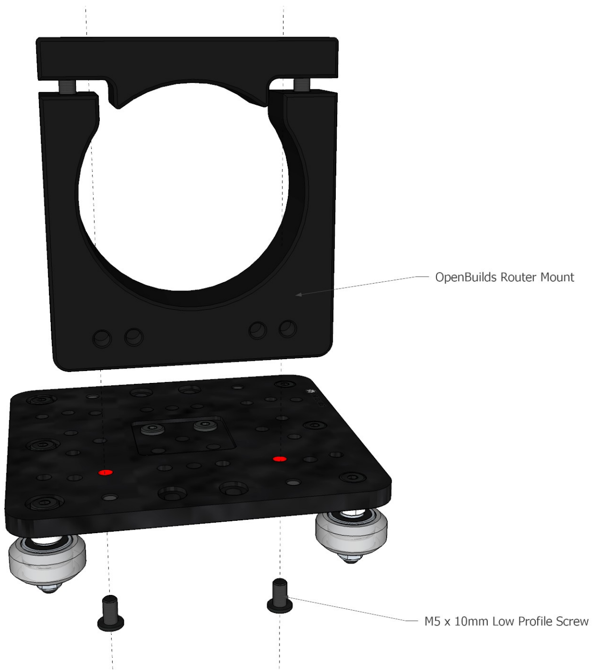
Figure 10: Assemble Z Axis Gantry Plate: Install Router Mount
