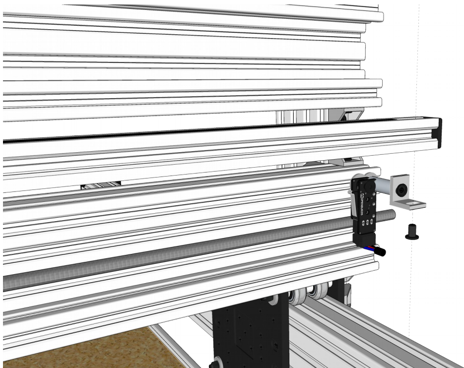
Figure 27: LEAD CNC Machine 1515 Disassembly: Remove Cable Chain Carrier
